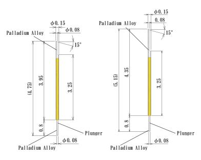
Preload 0.042N(4.3gf) 0.098N(10gf) at 0.45mm travel Full travel 0.6mm Current rating 0.3A Preload 0.042N(4.3gf) 0.098N(10gf) at 0.45mm travel Full travel 0.6mm Current rating 0.3A
